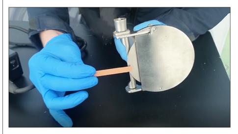
Turn the kebab knife on and allow the blade to spin. Apply light pressure to the top edge of the blade with the tool until sufficient sharpness is achieved.
